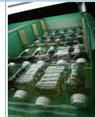
The experiment was carried out in 2.5 L PETG bottles incubated in a water bath at constant temperature and under artificial light conditions (16h-8h light-dark cycles).
